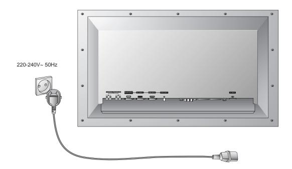
Your set must be connected to the mains through an earthed wall socket ( $\frac{1}{2}$ ). Use the delivered mains lead exclusively. Under no circumstances must an electrical extension lead be used.
